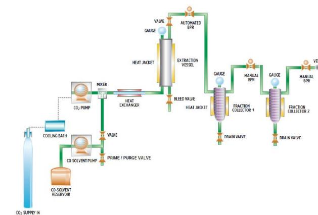
Figure 3. Representation of a supercritical CO<sub>2</sub> extractor.
