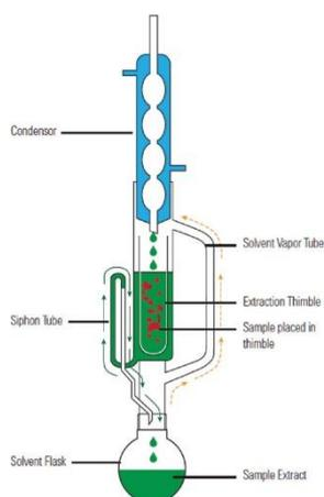
Figure 2. Representation of a Soxhlet apparatus.
