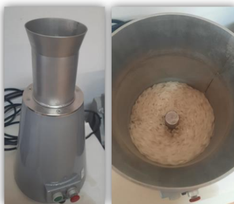
Figure 1 - Mixing Equipment (Ernesto Morgado, S.A.) to incorporate essential oil compounds in rice.
