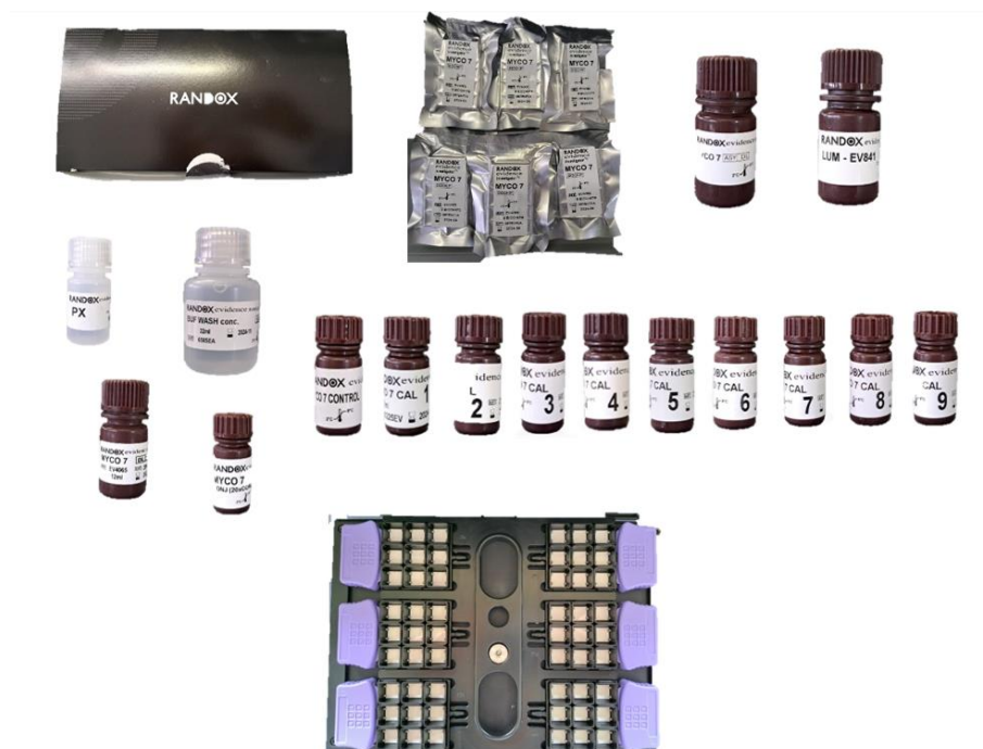
Figure 2. Components of the Myco 7 Array. Nine biochips, control, 9 calibrators, assay diluent, multianalyte conjugate, conjugate diluents, washing buffer and signal reagent.
