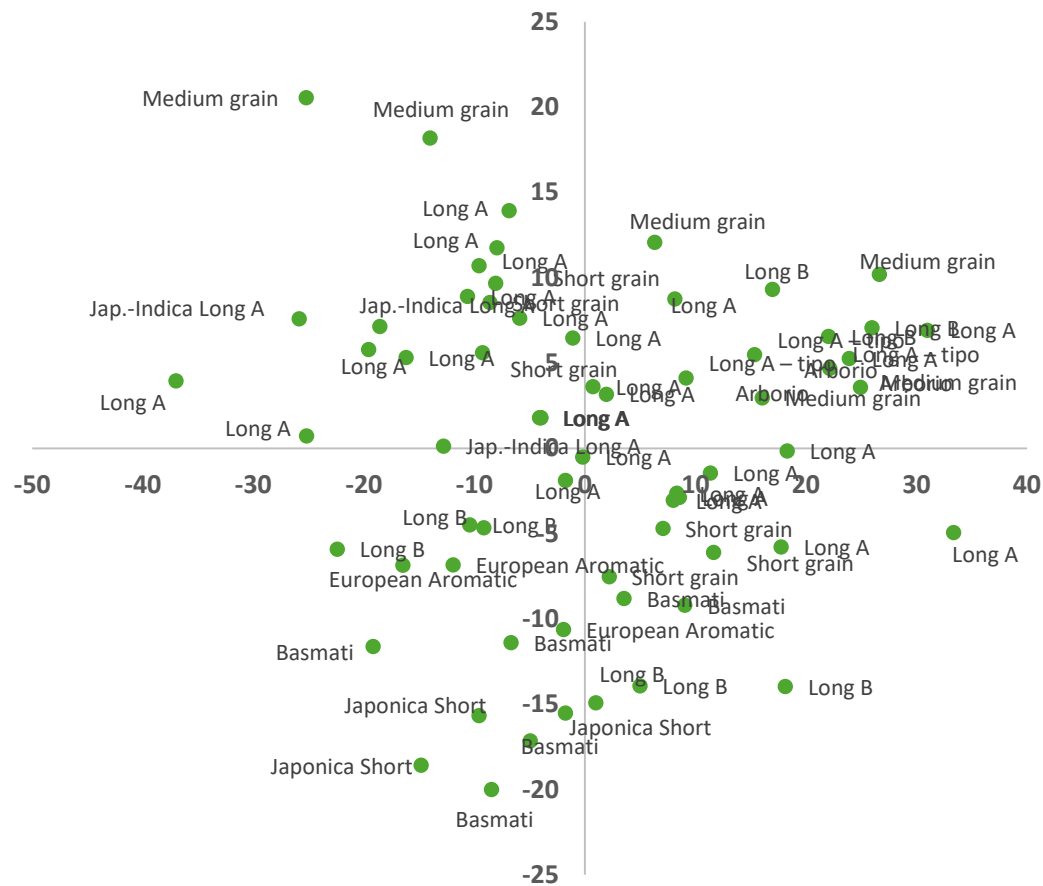
PCA based on NIR spectra obtained from flour
